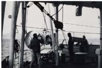
In 1965, the Surveyor used a sidescan sonar system to explore an offshore extension of the San Andreas Fault. (NOAA Photo Library). Click image for larger view.
